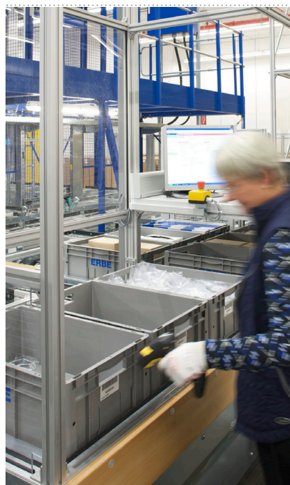
Laser-guided and visually supported picking in the automatic small-parts storage area
